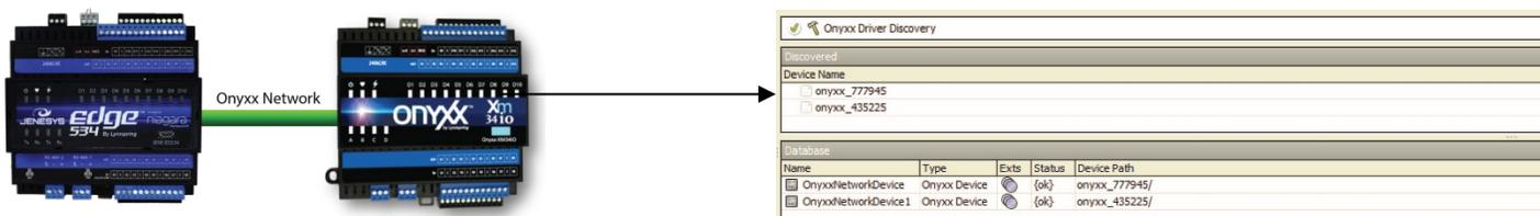
**Note:** Add to a JENE-EG534, up to 8 additional extender modules (*at 34 points of IO each*) for a maximum of 306 points.
